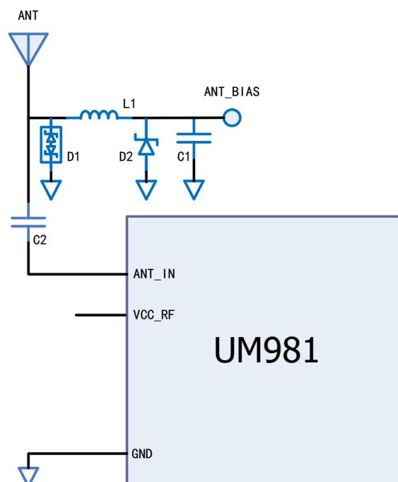
Figure 3-2 UM981 External Antenna Feed Reference Circuit
