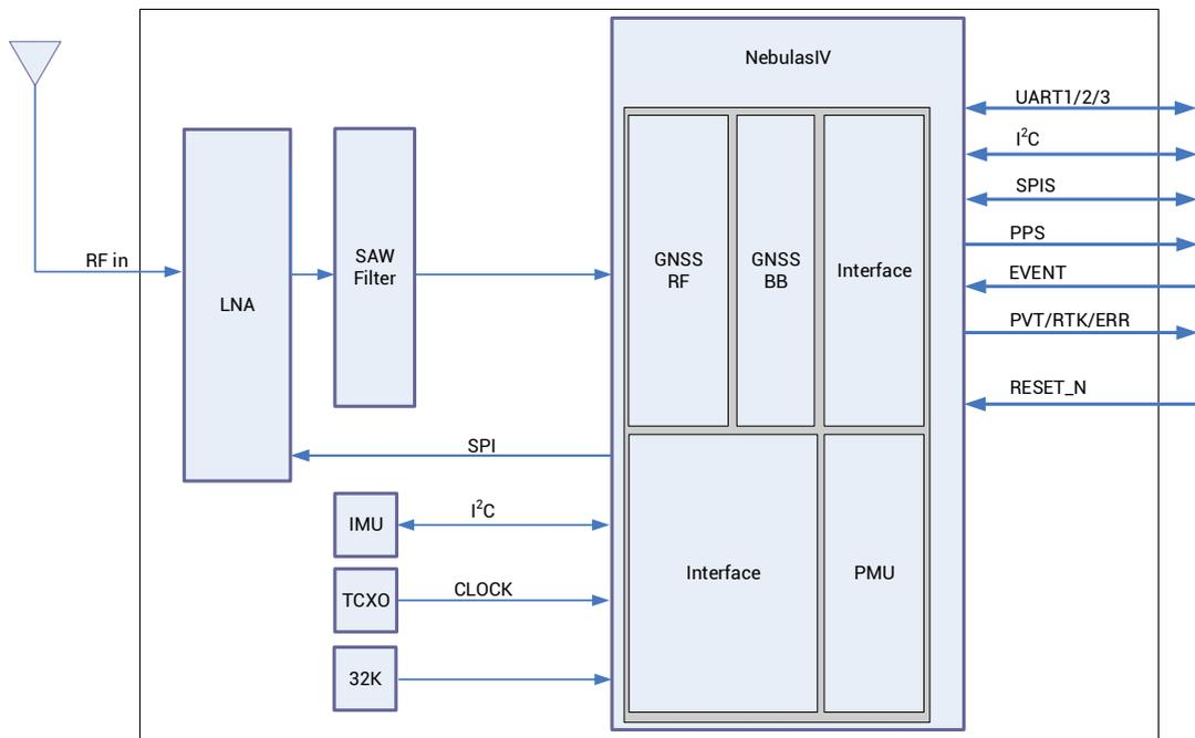
Figure 1-2 UM981 Block Diagram
